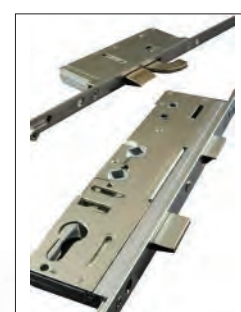
Yale The Mantis 3 Lock can be used with a Lever or Pad handle, the lock consists of ten locking points, four roller cams, two linear bolts, two hooks, a thumb latch and a dead bolt.
